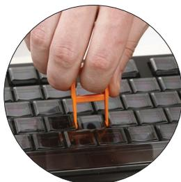
Bring the remover tool to the key holding it at a straight angle. Place the tongs astride the cap and push down until you hear a click.
