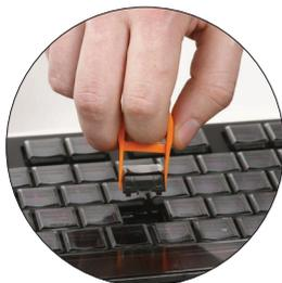
Pull the tool strictly vertically—holding it at a straight angle to your keyboard's surface, not to the table.
