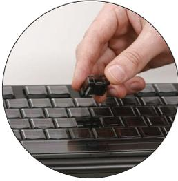
Position the key so that the main board pin contacts point into the slots in the display module, and the wider part is at the bottom, arranged towards the space bar.
