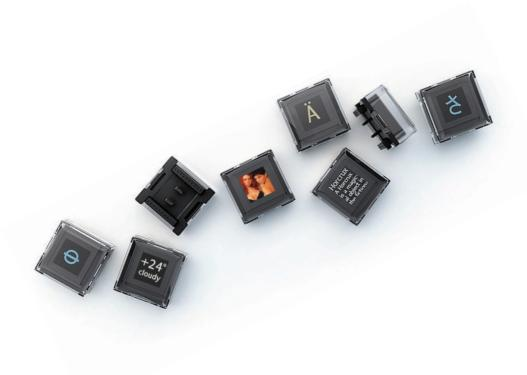
Optimus Maximus keys can be removed and replaced.
