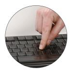
Once everything is correct, install the key by pressing the top of the cap down at the same angle.
