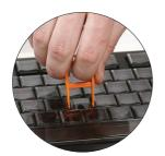
Bring the remover tool to the key holding it at a straight angle. Place the tongs astride the cap and push down until you hear a click.
