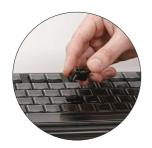
Position the key so that the main board pin contacts point into the slots in the display module, and the wider part is at the bottom, arranged towards the space bar.
