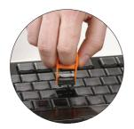
Pull the tool strictly vertically—holding it at a straight angle to your keyboard's surface, not to the table.
